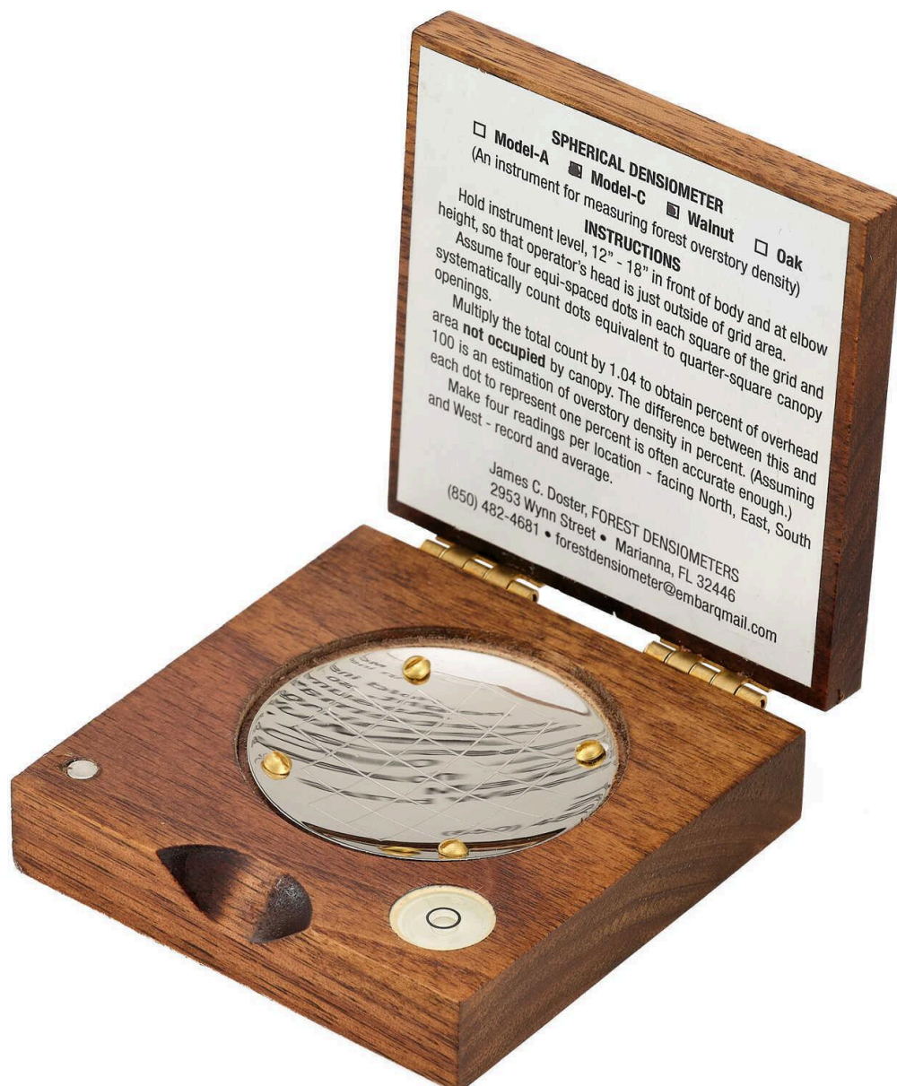
Figure 13: Densiometer, used to measure canopy density at every camera location
